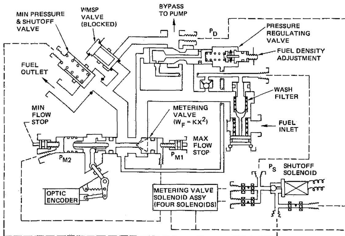
Figure 10 Schematic of Fuel Flow Package
