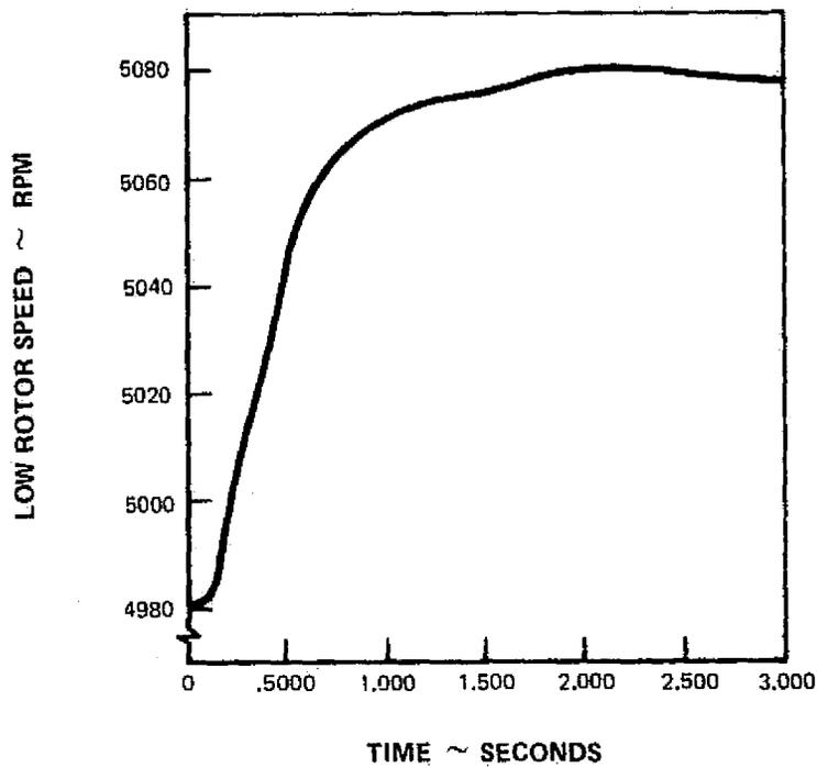
Figure 20 Response of the Two-Solenoid Digital Effector with 12-bit Position Feedback Resolution to Small Power Lever Step at Sea Level Static, High Power
