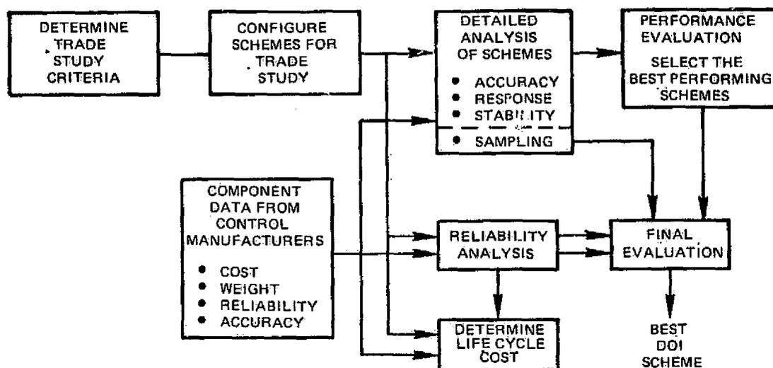
Figure 2 Digital Output Interface Trade Study Procedure
