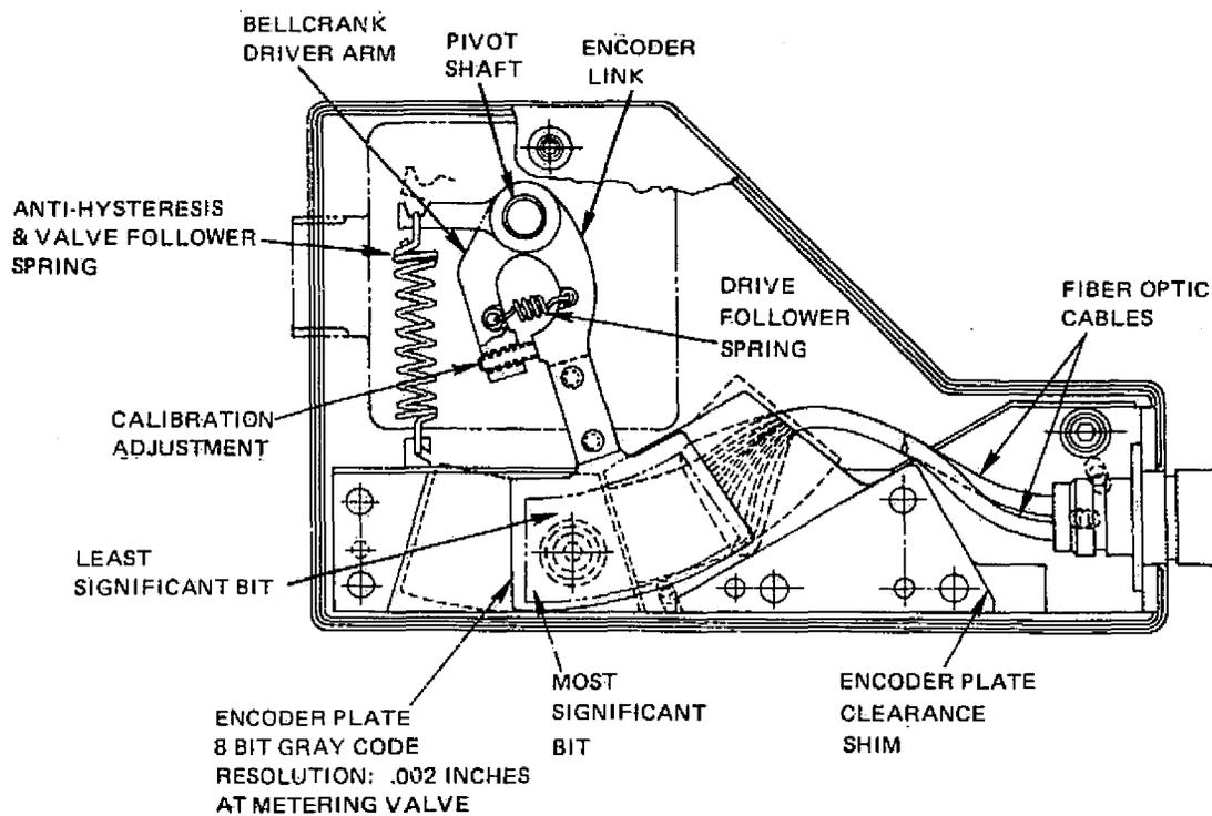
Figure 9 Schematic of Optical Position Sensor
