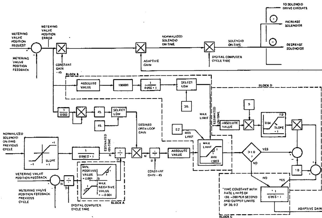
Figure 16 Block Diagram of the Adaptive Logic
