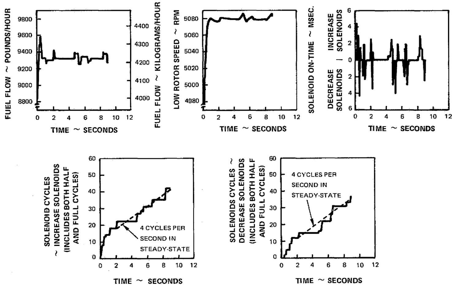
Figure 18 Small Power Lever Step and Steady-State Operation at Sea Level Static, High Power with the Two-Solenoid Configuration and with Revised Adaptive Logic
