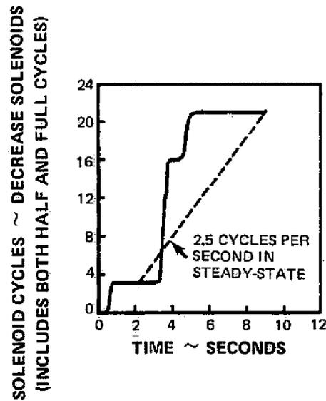
Figure 23 Small Power Lever Step and Steady-State Operation at Sea Level Static, High Power with the Four-Solenoid Configuration
