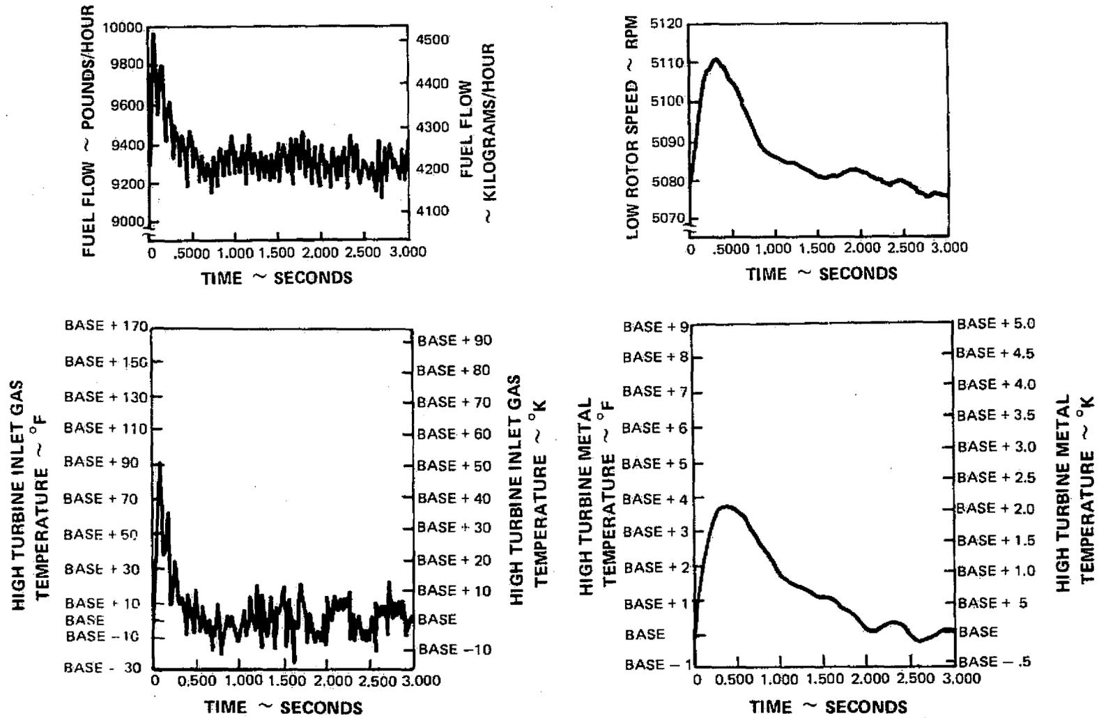
Figure 25 Response Due to One Increase Solenoid Failing Open at Sea Level Static, High Power
