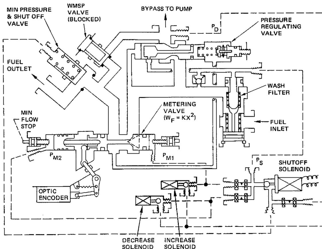
Figure 6 Two-Solenoid Configuration
