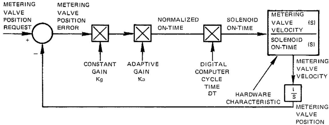
$$(B1) \text{ OPEN LOOP GAIN} = K_g \cdot K_a \cdot \frac{\text{METERING VALVE VELOCITY}}{(\text{SOLENOID ON TIME})} \cdot DT$$
