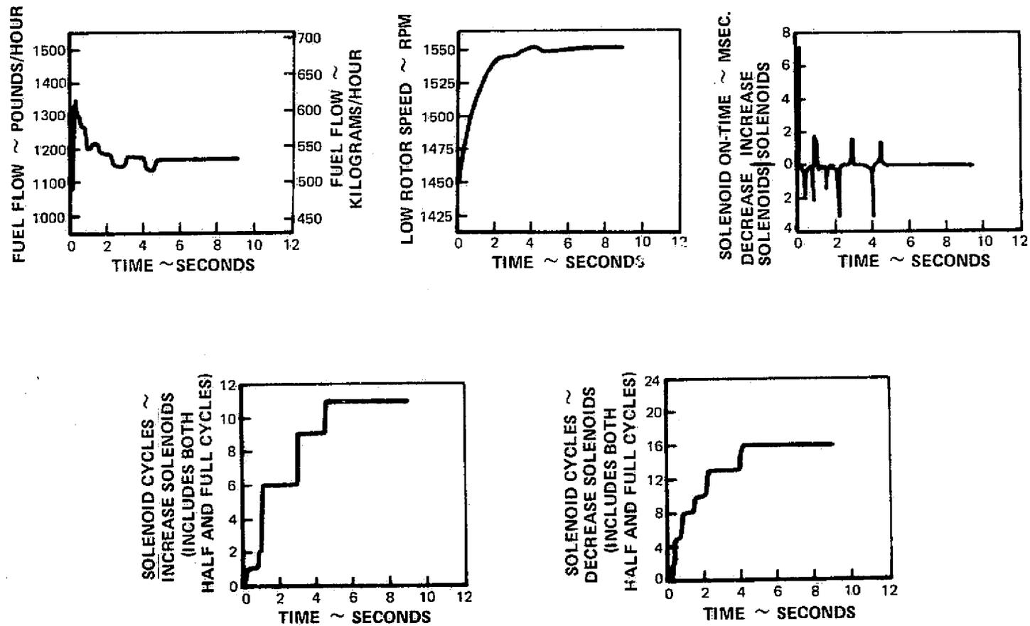
Figure 24 Small Power Lever Step and Steady-State Operation at Idle with the Four-Solenoid Configuration and with Reduced Loading from the Optical Encoder
