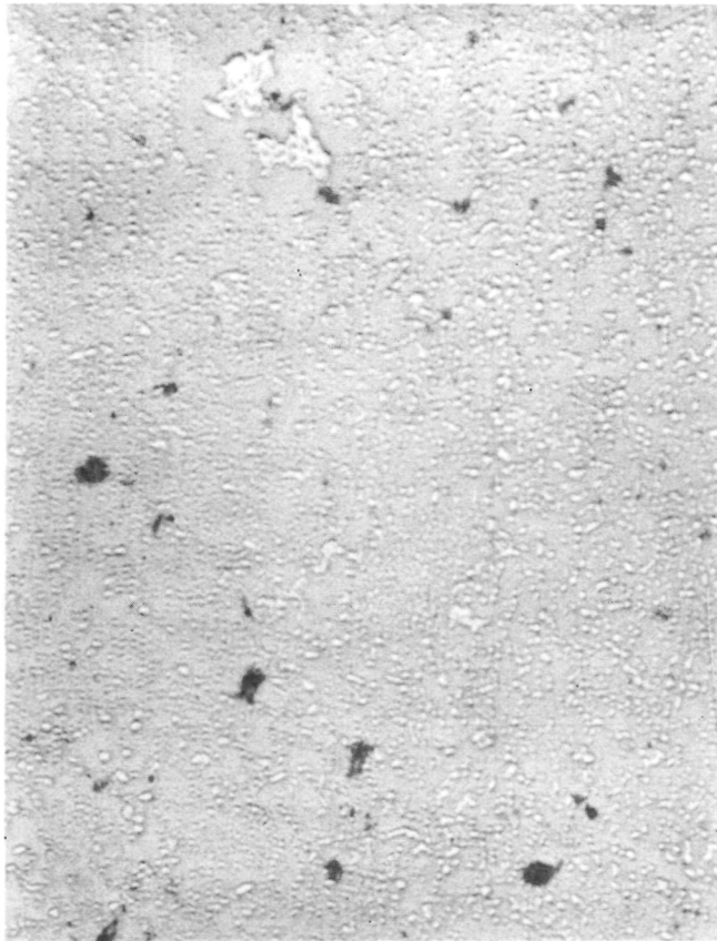
Figure 1. - Microstructure of hot pressed Ni-Cr-Al-Y powder. White phase is \gamma . Etched; X750.
