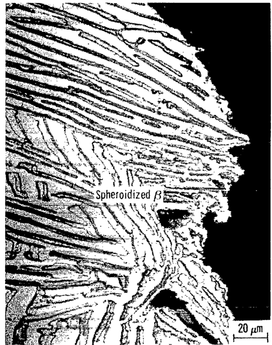
(c) Temperature, 1100°C (Light micrograph, longitudinal section).
