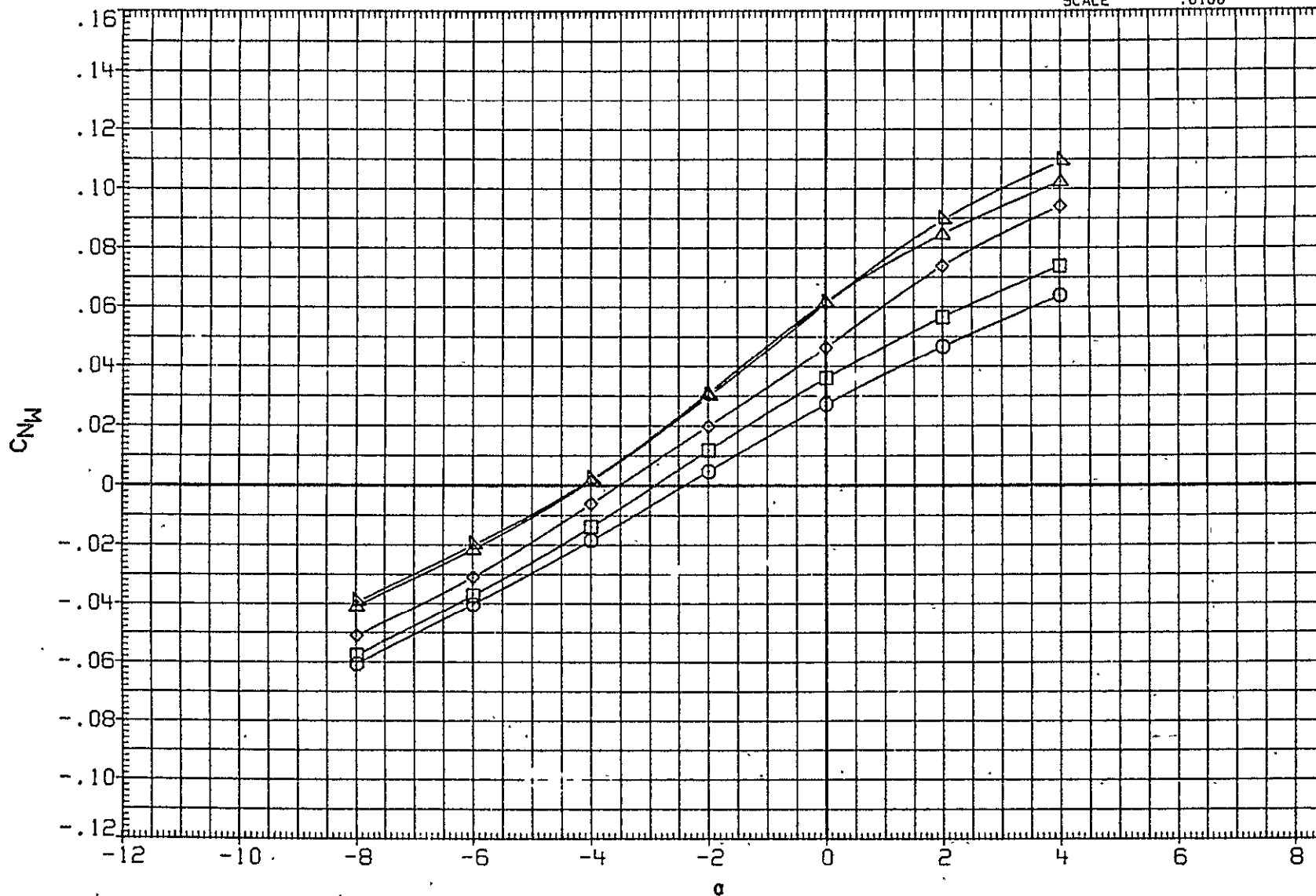
FIG. 6 ORBITER WING SHEAR, BENDING, AND TORSION COEFFICIENTS
