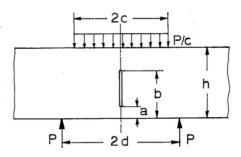
Figure 1. Geometry for a cracked strip under bending.
