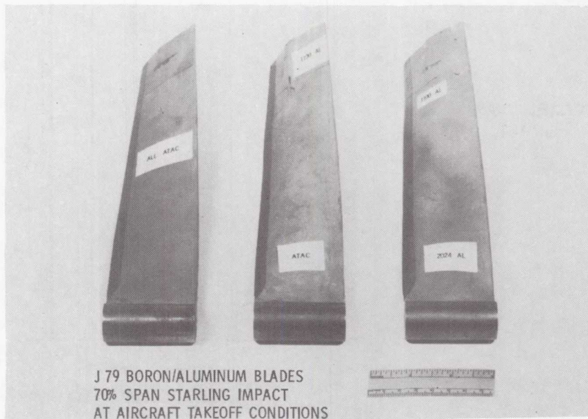
Figure 8.- J-79 boron/aluminum blades after bird impact testing at takeoff conditions. (Starling impact at 70 percent of span.)
