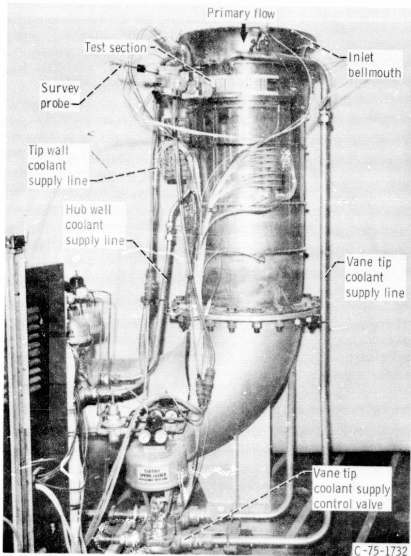
Figure 1. - Core-turbine stator annular cascade.
