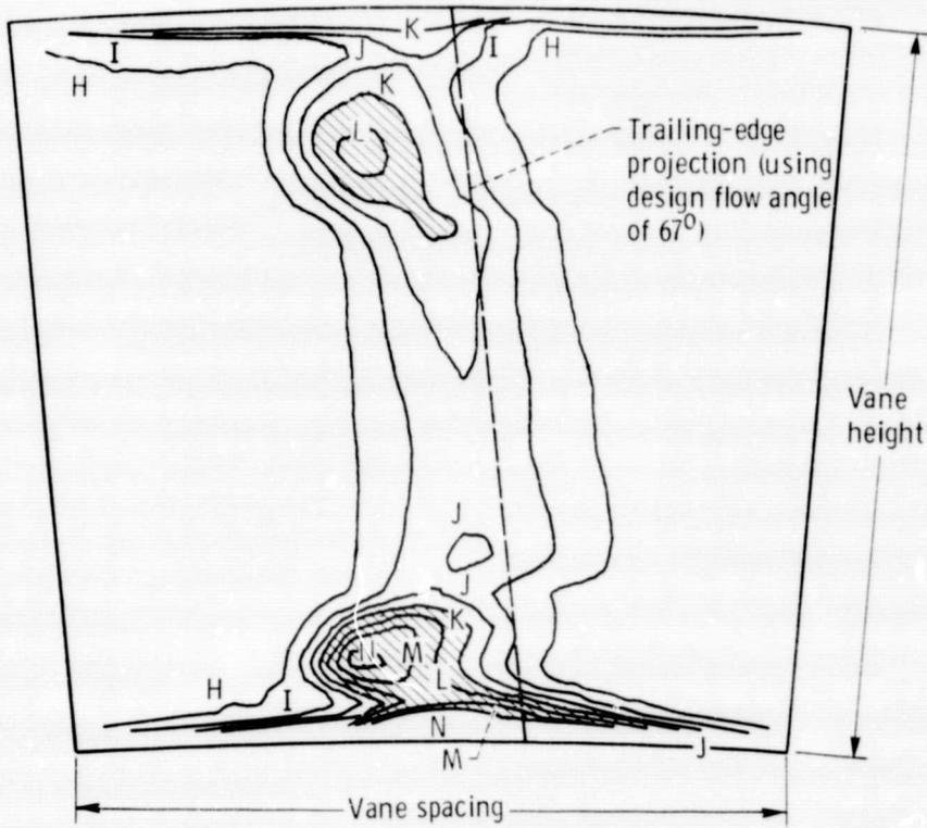
(c) Coolant to inlet total-pressure ratio,  $p_c'/p_0'$ , 1.4.
