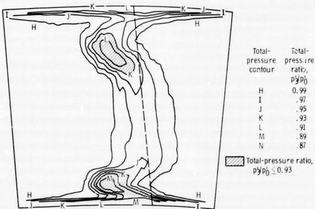
(b) Coolant to inlet total-pressure ratio,  $p_c^0/p_0^0$ , 1.0.
