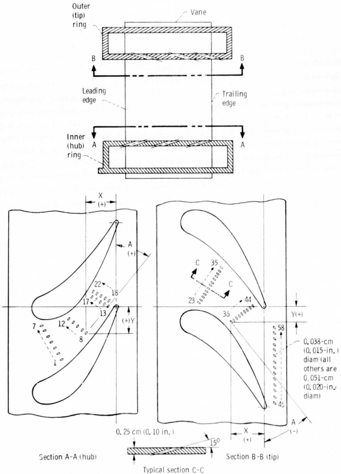
Figure 5. - Schematic of endwall cooling geometry.
