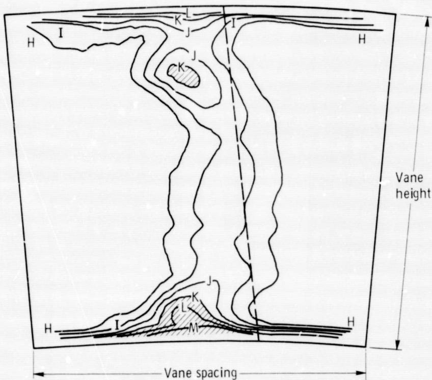
(c) Coolant to inlet total-pressure ratio,  $p_c^i/p_0^i$ , 1.4.
