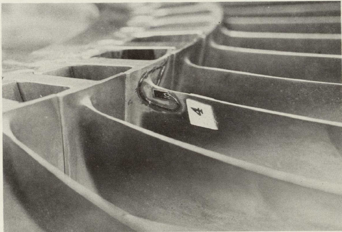
Figure 39. Actual Gauge Installation Locations on the 20-Inch Fan Rotor Disk and Blades.
