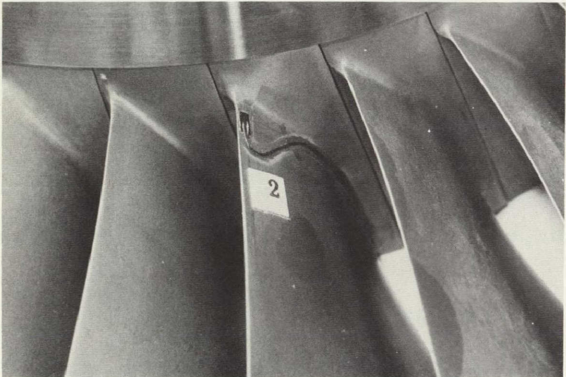
Figure 38. Actual Gauge Installation Locations on the 20-Inch Fan Rotor Disk and Blades.
