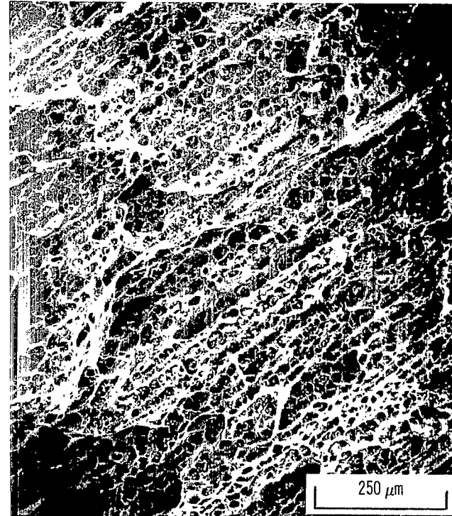
(b) Creep-tested at 1365 K and 18.9 MPa for 148.7 hours with 0.44 percent strain.
