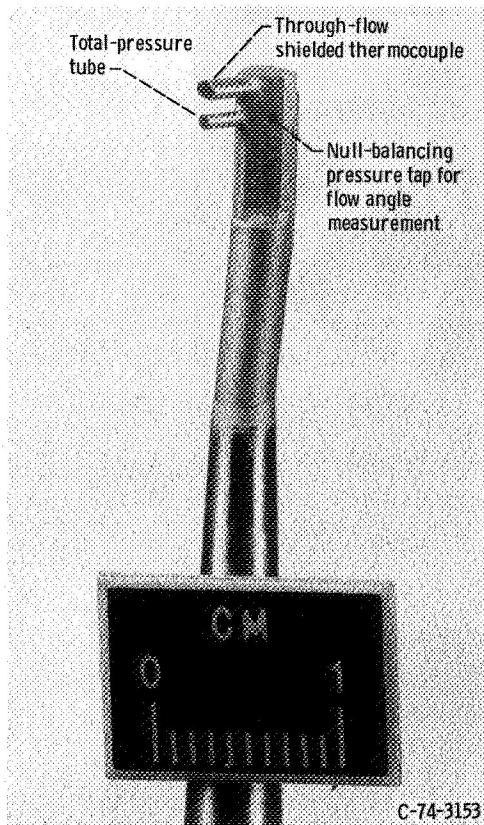
(a) Combination total pressure, total temperature, and flow angle probe.
