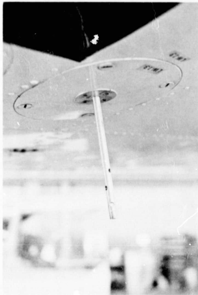
Figure 12. Wing Installation of Outside Air Temperature Probe
