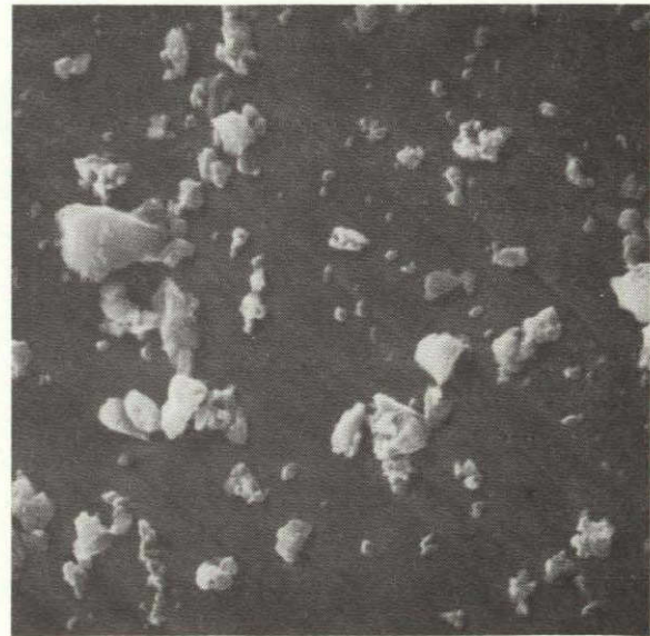
Magnification 3000 x After Ball Milling
