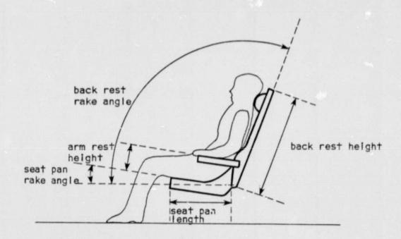
Figure 1. Typical Passenger-Seat Configuration
