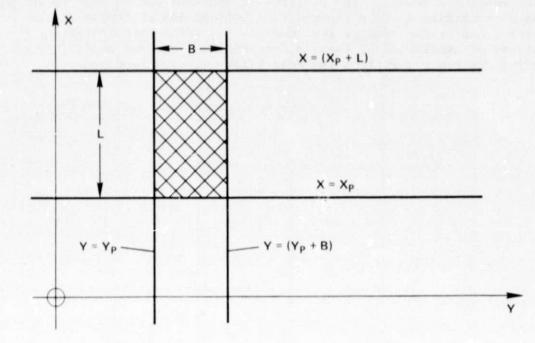
In this case, the aircraft will be over the landing platform when the following geometrical conditions are met:
