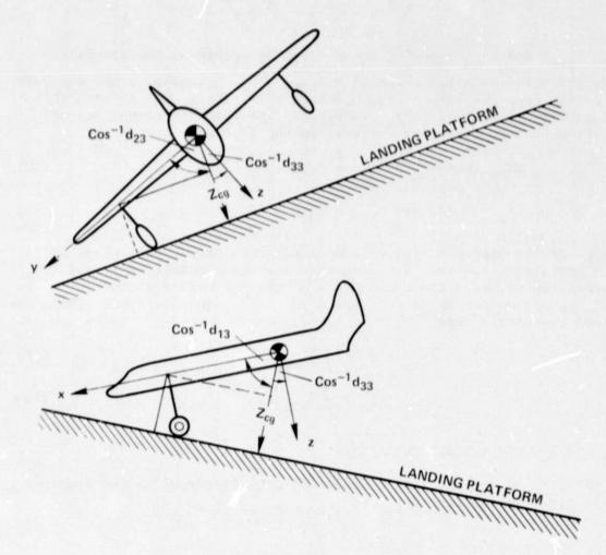
Equations (24) through (26) give the components of aircraft velocity relative to the landing platform. These are referred to aircraft body axes. In order to determine the corresponding components in ship axes, the aircraft velocity components must be transformed to ship axes. Subsequent to transformation, equation (24) assumes the form
