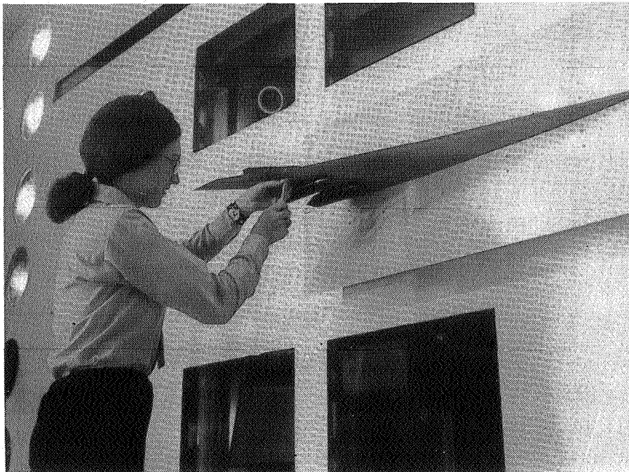
Figure 8.- Photograph of arrow-wing model mounted in wind tunnel.
