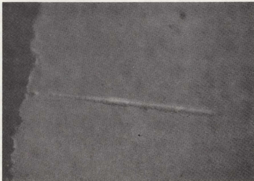
Figure 43. Facet damage observed on high-power LOC laser at the 1200-W/cm operating level. (Facet originally coated with SiO which was removed to obtain this photograph.)
