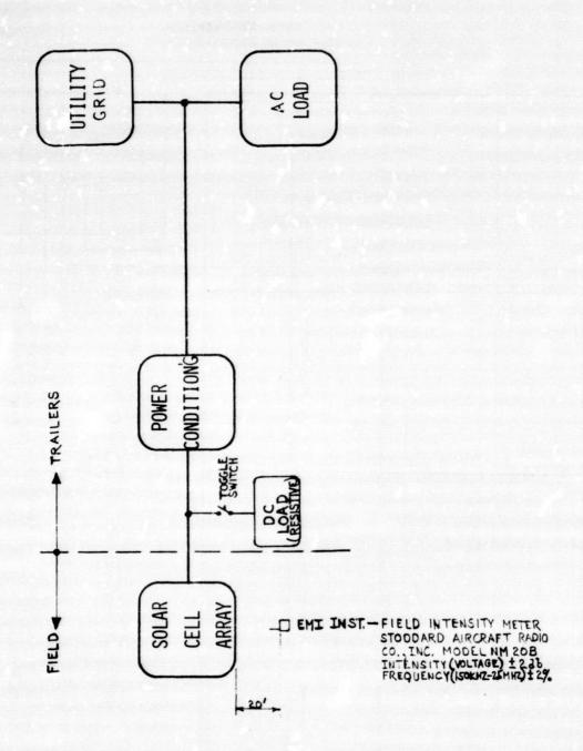
FIGURE 4 SIMPLIFIED BLOCK DIAGRAM FOR EMI TEST SET-UP
