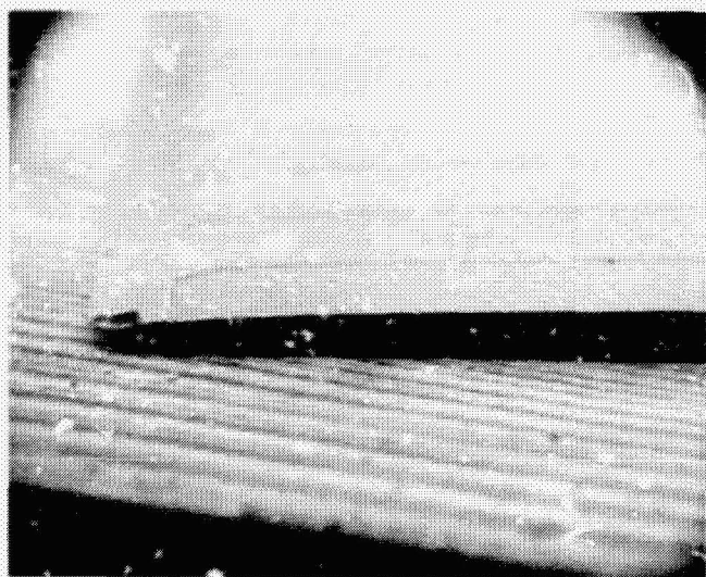
Fig. 7. Edge view of bare Ferranti cell presenting its pronounced etched taper; SEM, 65x
