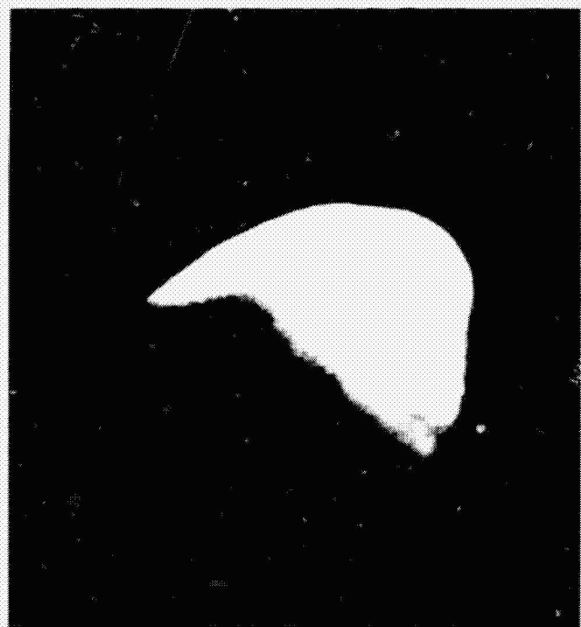
Fig. 24. Top of a carrot defect on RF sputtered DC 7070 film; SEM, 1540 \times (from Ref. 2)
