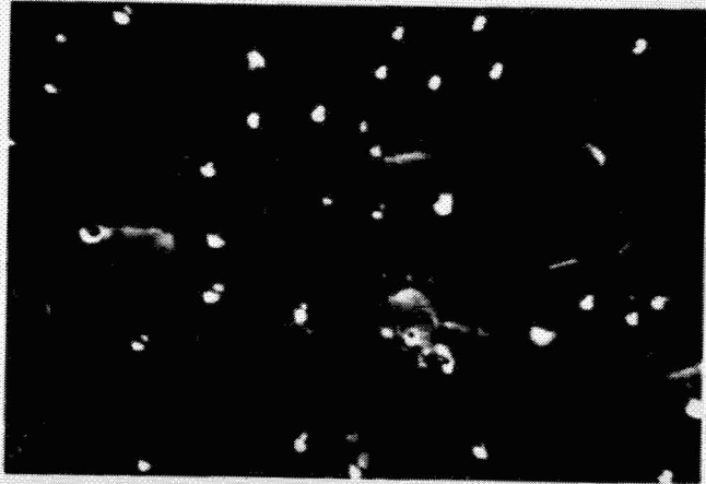
Fig. 20. The bright objects are carrot defects; SEM, 670 \times . Etched patterns on the solar cell surface are the larger features (from Ref. 3)
