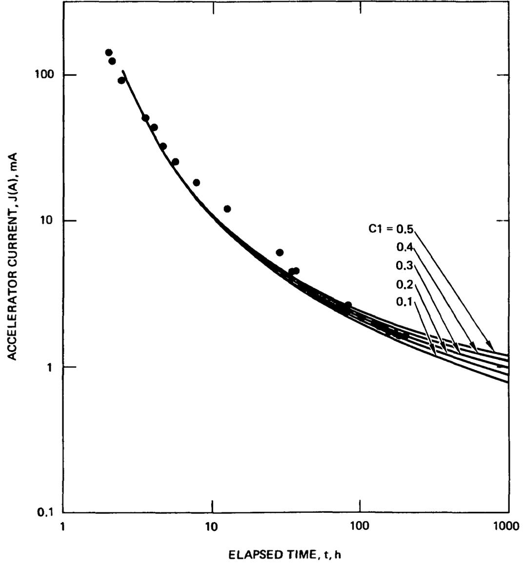
Figure B-1. Analytical expression  $\overline{J(A)}$  plotted as a function of the curve-fitting parameter  $C_1$ .
