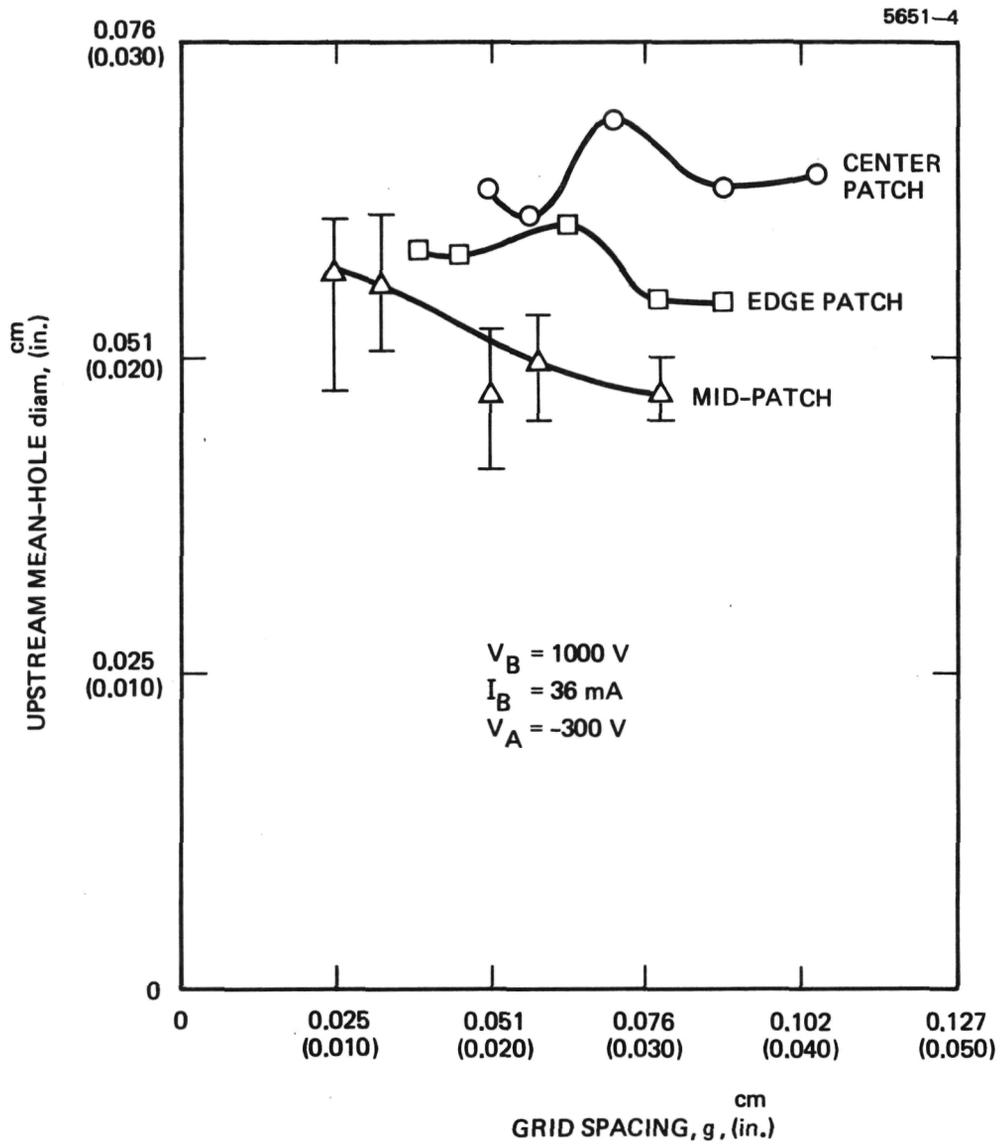
Figure 16. Upstream mean hole diameter versus interelectrode spacing for beam current  $I_B = 36 \text{ mA}$ . Edge patch asymmetries are indicated by error bars.
