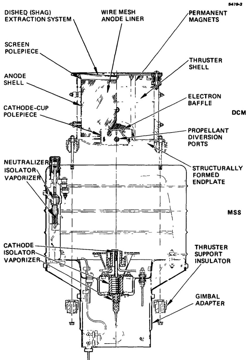
Figure 1. Attachment of discharge chamber module (DCM) to module support system (MSS).
