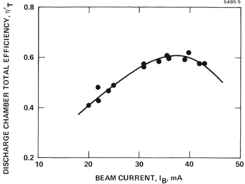
Figure 8. Discharge chamber total efficiency,  $\eta'_T$  as a function of beam current,  $I_B$ , for 0.5 mlb optimized DCM.
