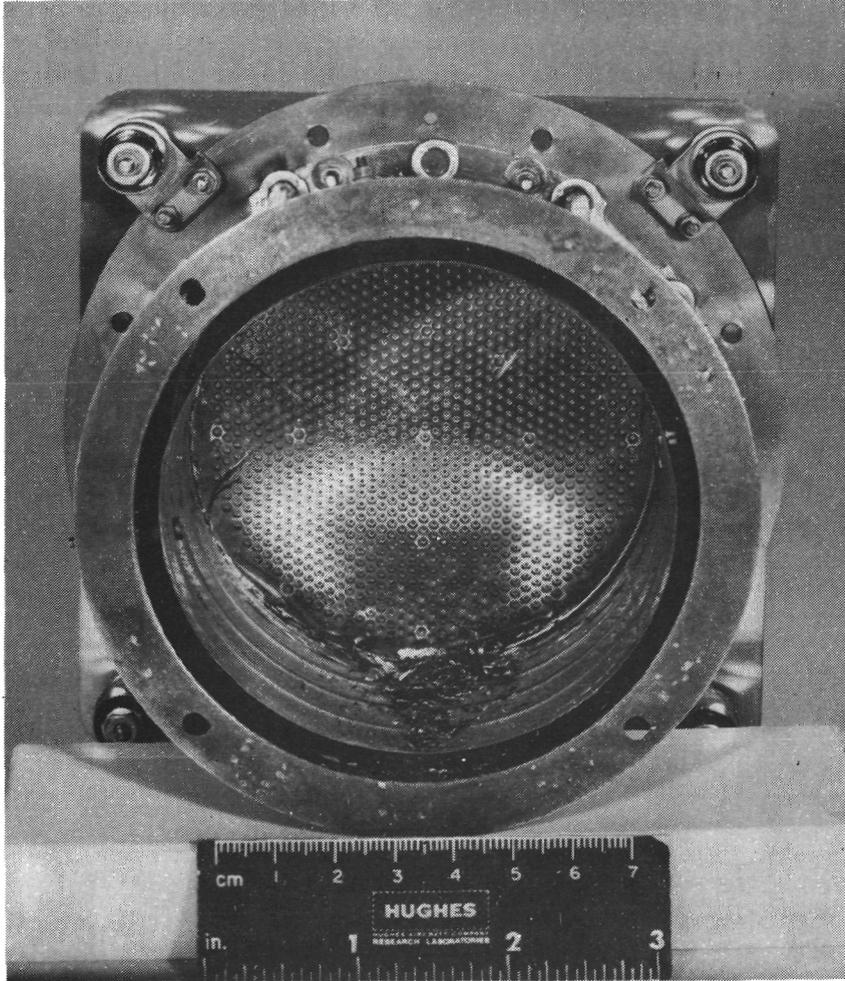
Figure 23. Discharge chamber after 200 hour test (0.5 mlb).
