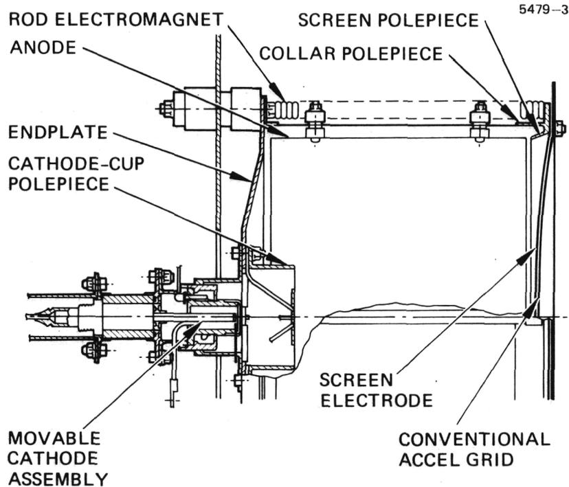
Figure 5. Versatile thruster assembly for optimization testing.
