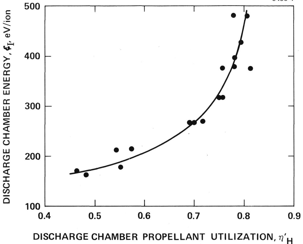
Figure 7. Discharge chamber energy,  $\mathcal{E}_i$ , as a function of discharge chamber propellant utilization,  $\eta'_{Hg}$  for 0.5 mlb optimized DCM.
