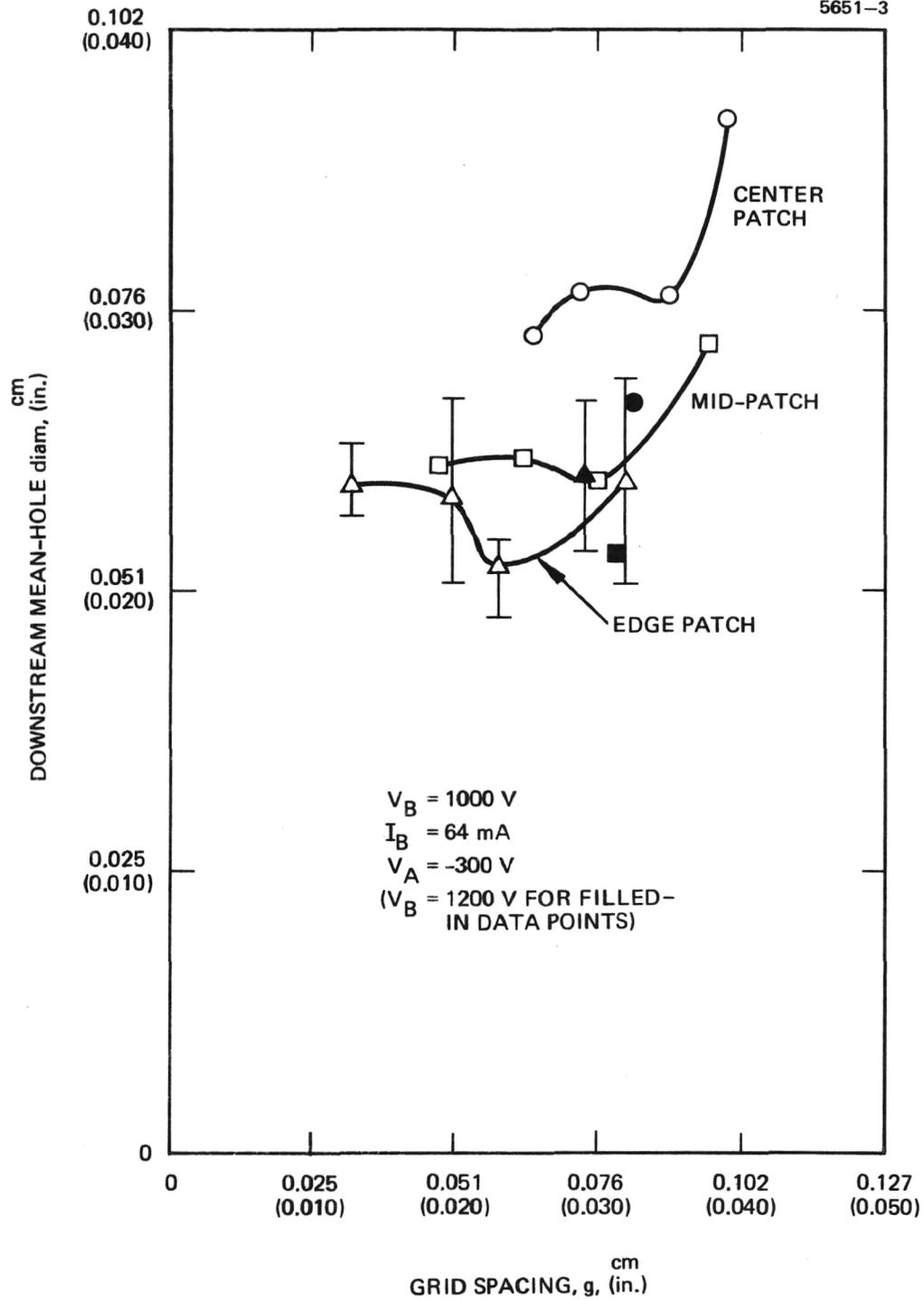
Figure 15. Downstream mean hole diameter versus interelectrode spacing for beam current  $I_B = 64 \text{ mA}$ . Edge patch asymmetries are indicated by error bars.
