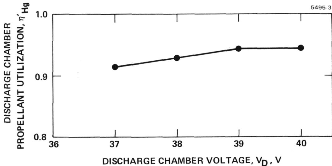
Figure 13. Discharge chamber utilization,  $\eta_{Hg}^i$ , as a function of discharge chamber voltage,  $V_D$ , for 2.0 mlb optimized DCM.
