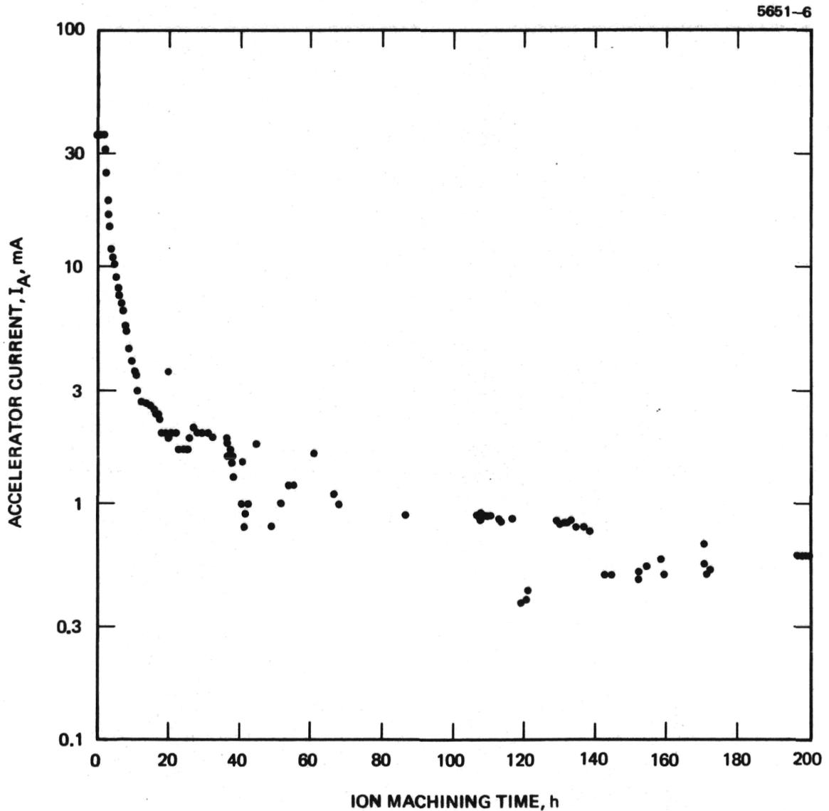
Figure 20. Accelerator current versus time for 0.5 mlb DCM.
