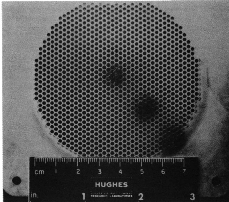
Figure 18. Upstream view of accel and PT-3 patches.
