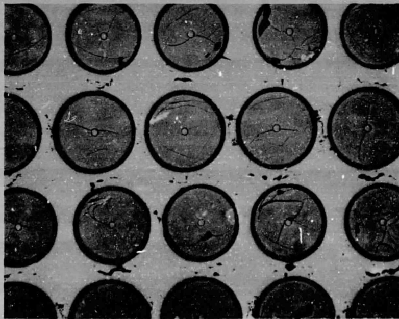
Figure 13. - Micrograph of typical 203 \mu\text{m} B-6061 Al specimen after thermal cycling 3000 times to 320° C.
