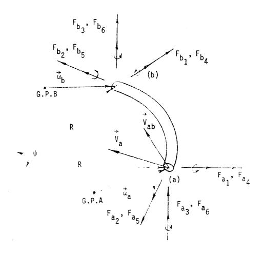
Figure (4). - Element Forces and Geometry.
