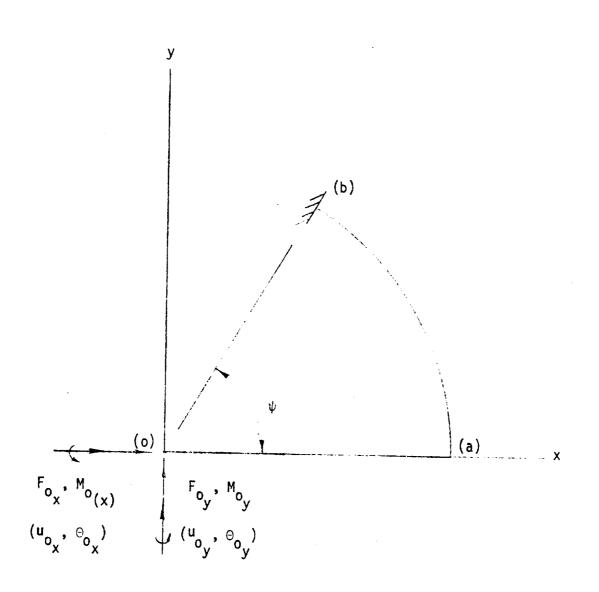
Figure (1). - Geometry and Notation for Chen Flexibility Matrix
