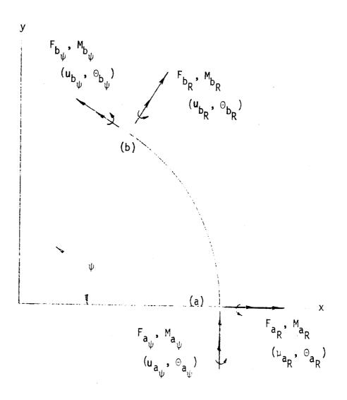
Figure (2). - In Plane Forces and Displacements for the Curved Pipe Element.
