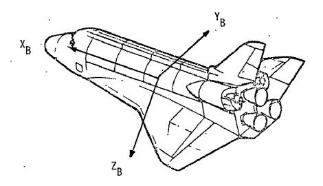
System 1 is the longeron system, which is fixed in the longeron supporting the arm. The x-axis or 1-axis is positive aft, the z-axis is downward and perpendicular to the longeron, and the y-axis is to the left, completing the right-hand system. This system is rolled outboard through an angle  $\phi$  during RMS deployment activity. The transformation matrix from the body system to the longeron system can be written as
