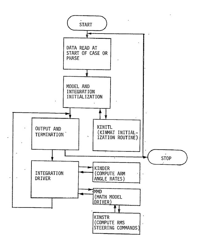
Figure 1.- Overview of SVDS with KINMAT interfaces.
