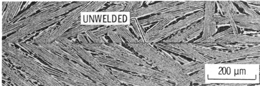
Figure 5. - Transverse section of lap joint diffusion weld in \gamma/\gamma'-\delta bar showing unwelded region.
