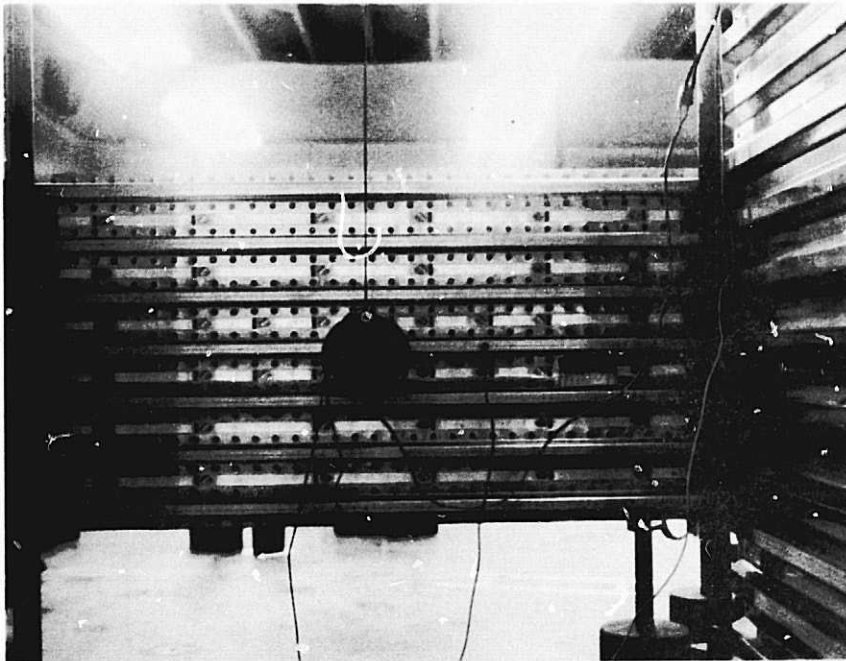
Figure 5. Experimental Configuration Used for Producing Holograms of the Space Shuttle Test Panel.
