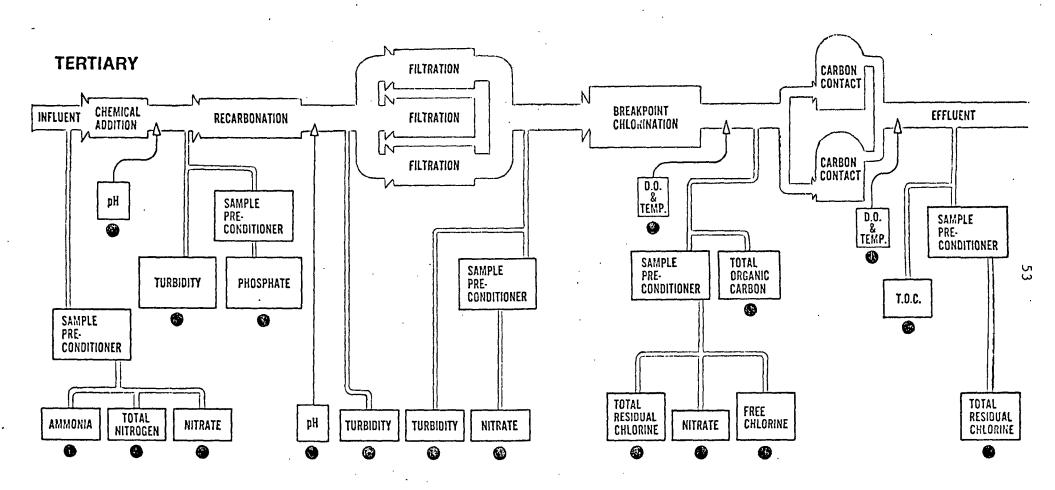
FIGURE 1. SCHEMATIC DIAGRAM OF A HYPOTHETICAL TERTIARY TREATMENT PROCESS INDICATING MONITORING POINTS (DELTA SCIENTIFIC) (5)
