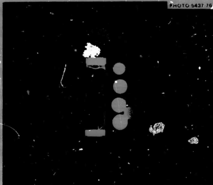
Figure 16. A print from an autoradiograph of ground base sample 13-B. Note the Au activity in the grain boundary. The Pb sample is fairly dark because the Au concentration is low and is fairly uniform over the sample.
