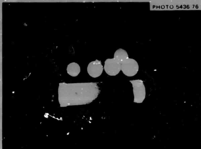
Figure 15. A print from an autoradiograph of space flight specimen 12-B. The wetted mild steel ampoule can be seen. The light areas in the end caps do not represent Au activity, but other activities that are the result of the thermal neutron irradiation of the mild steel ampoule. The light area in the Pb does represent Au activity.
