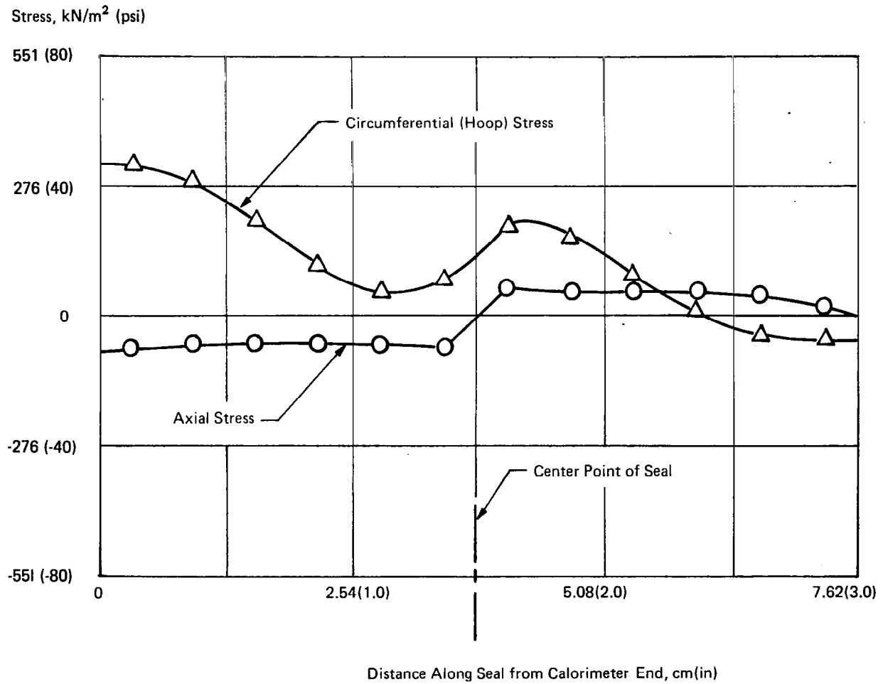
Figure 45. Thermal Membrane Stress Distribution in Calorimeter Seal at 20,000 Seconds after Emptying
