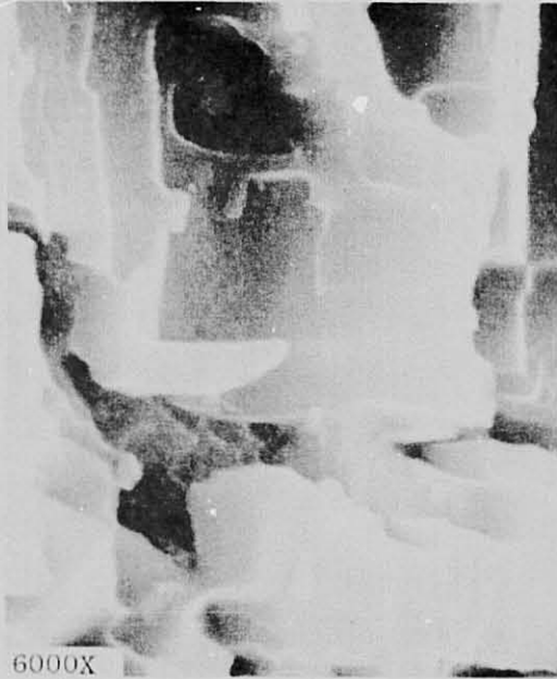
Figure 26. Extent of 0.002 inch 1100 Al Surface Attack with S/F 15 Preparation. SEM at 45°.
