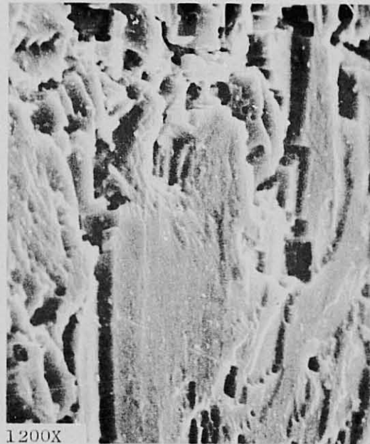
Figure 26. Extent of 0.002 inch 1100 Al Surface Attack with S/F 15 Preparation. SEM at 45°.
