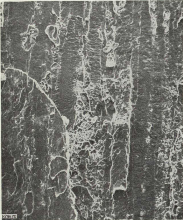
Figure F4. Stress corrosion fracture surface on SL-DCB specimen from 1.25-in. 7075-T7351 plate: salt-chromate environment (45°)
