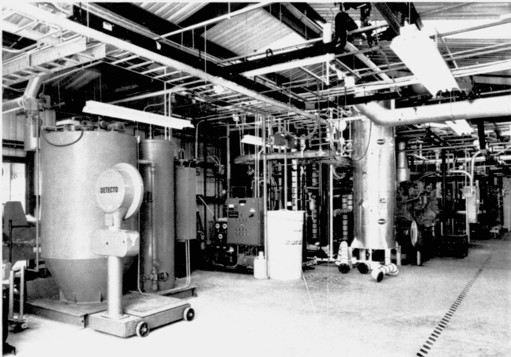
Figure 1.- Hamilton Standard test article for the MIST, showing piping and integrated hardware (NASA S-74-23335).
