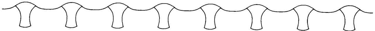
Figure 7.- Local buckling mode shape for panel whose buckling response diagram is shown in figure 5. \lambda = L/28 .
