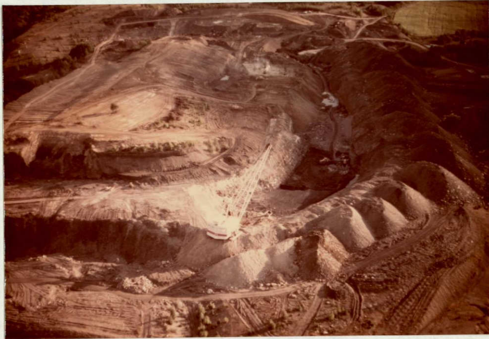
Figure 3. This aerial view of Clarion County, Pennsylvania illustrates a typical strip mining operation for coal. The drag line in the foreground removes the earth overlying the coal bed and piles it to one side of the open trench. The coal is loaded onto trucks by power shovels or, as in this photograph, by large front-loaders. Drilling in the center-background is for blasting to break and loosen the rock strata so that drag line can remove it. As that loosened rock is removed, it will be piled in the existing trench. Thus, the elongate trench and highwall will move to the left across the area. The rock material pile on the right will be leveled to the approximate original contour of the land. The top soil, which was removed and stock piled prior to mining, will be replaced after regrading. The land will then be revegetated as forest-grassland or developed as farmland.
