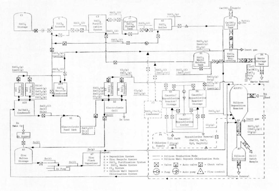
FIGURE 1. PROCESS FLOW DIAGRAM FOR 25 MT/YEAR SILICON FACILITY (7/5/77)
