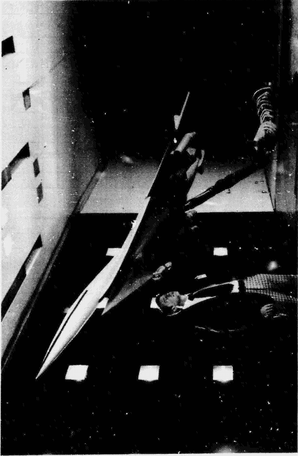
Figure 3. - Photograph of model mounted for tests in Langley V / STOL tunnel.
