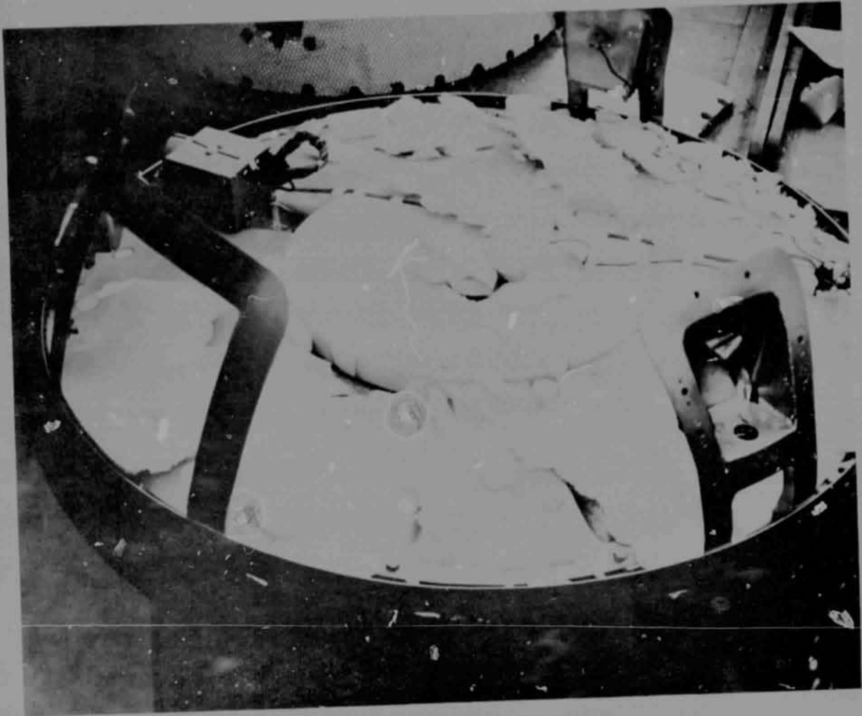
AFT FOAM INSULATION AFTER THERMAL VACUUM TEST
