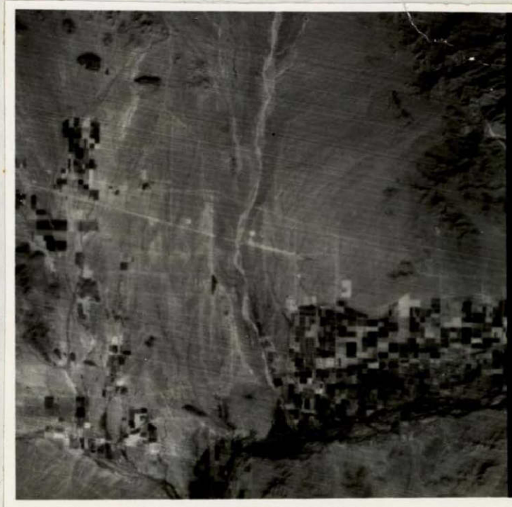
Figure 11. Repetitive ERTS coverage shows construction progress between May and October 1973 on Interstate 10 west of Phoenix. The highway is a white line extending southeastward from the left edge of the photo. In the later (October) ERTS image (below), it has crossed the Hassayampa River.
