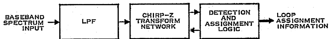
Figure 4-5. Block Diagram of a Single-Ensemble Chirp-Z Transform Frequency-Determining Circuit
