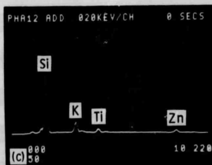
Figure 5. - (a) Electron micrograph of wear debris from test F-7 (98 hours), (b) energy dispersive x-ray analysis (EDAX) of particle A, (c) background EDAX of ferrogram.
