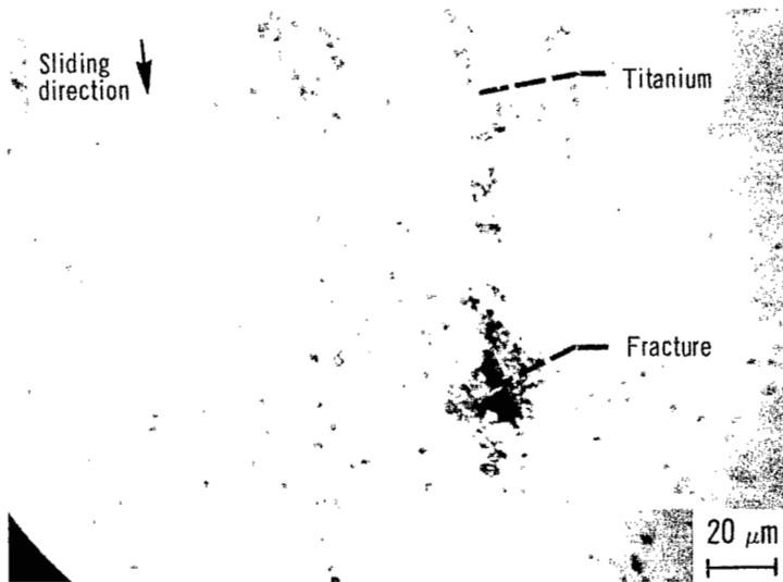
Figure 7. - Adhesion of titanium to smooth silicon carbide surface. Sliding velocity, 3 mm/inin; load, 50 grams; temperature, 25° C; environment, argon; pressure, atmospheric. (Fracture occurs in silicon carbide.)
