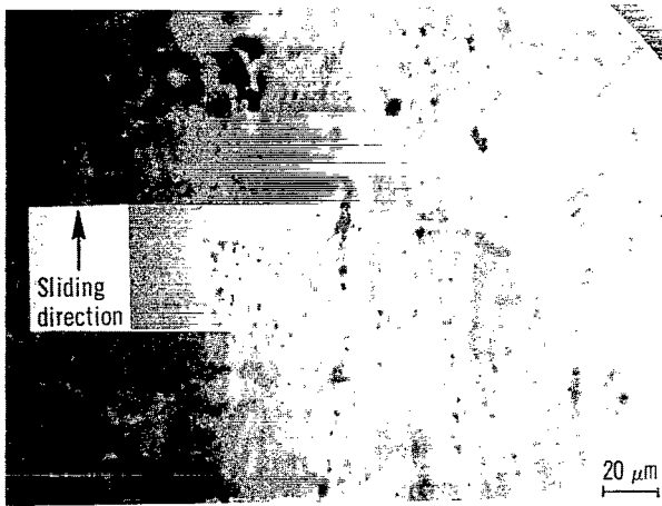
Figure 15. - Adhesion of titanium to smooth silicon carbide surface. Sliding velocity, 0.7 mm/min; load, 40 grams; temperature, 25° C, pressure, 10^{-8} N/m 2 .
