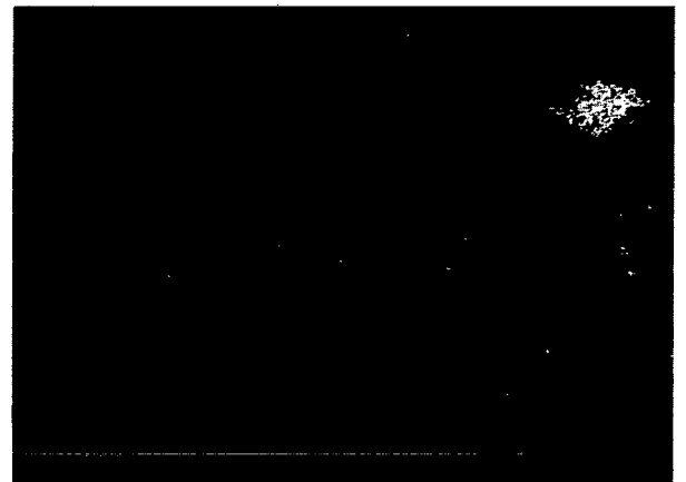
(b) Silicon K_{\alpha} X-ray map of titanium rider; 5 \times 10^3 counts.
