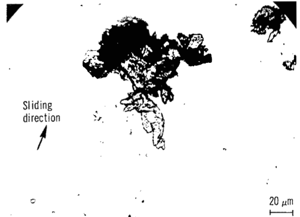
Figure 20. - Wear tracks on smooth silicon carbide surface. Sliding velocity, 0.7 mm/min; load, 40 grams; temperature, 25° C; pressure, 10^{-8} N/m 2 .
