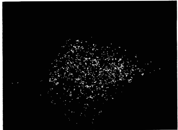
(b) Silicon K_{\alpha} X-ray map; 5 \times 10^3 counts.
