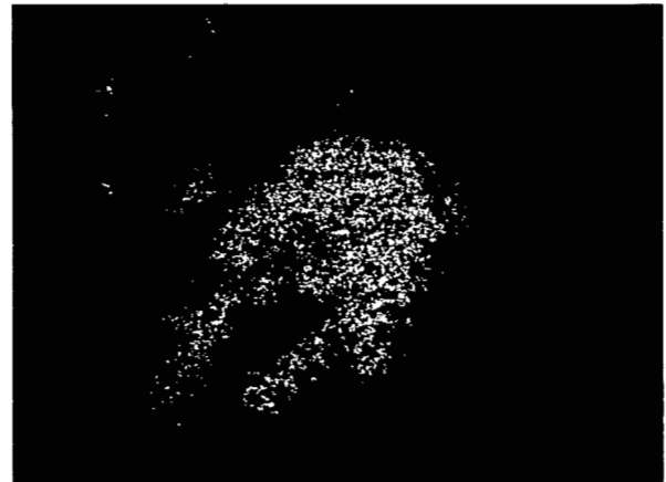
(b-2) Titanium K_{\alpha} X-ray map of silicon carbide surface; 5 \times 10^3 counts.
