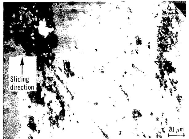
Figure 15. - Adhesion of titanium to smooth silicon carbide surface. Sliding velocity, 0.7 mm/min; load, 40 grams; temperature, 25° C, pressure, 10^{-8} N/m 2 .
