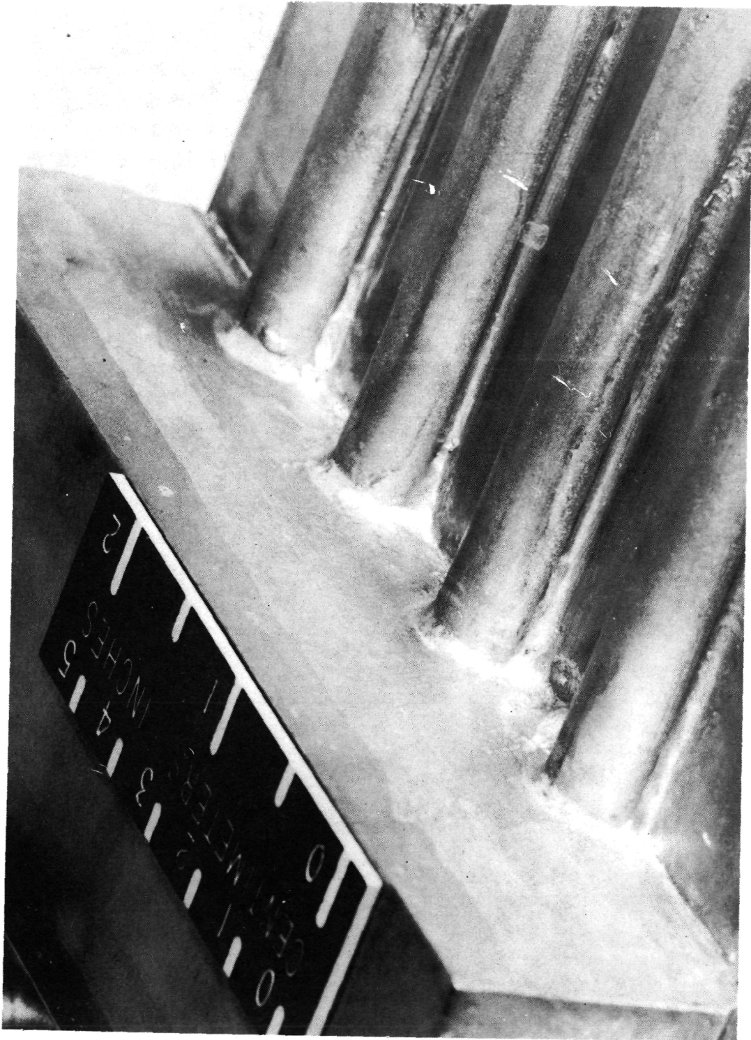
(c) Close-up of soldered tubes and brazed manifold-tube joints.
