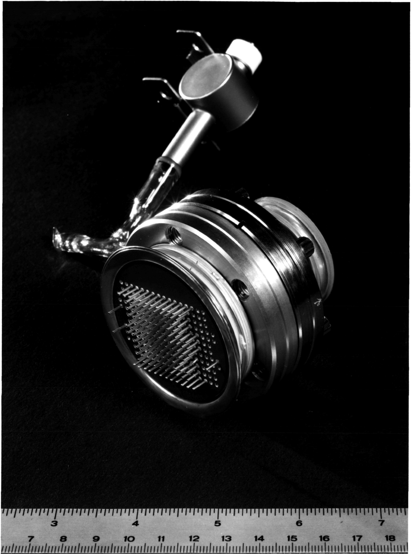
Figure 17. Demountable tube assembly incorporating type I multi-layer ceramic header.
