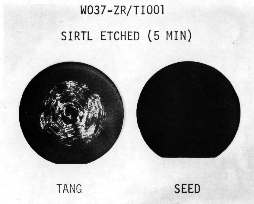
Fig. 28. Typical cellular structure which developed toward the end of a Zr/Ti-doped silicon crystal grown at 6.9 cm/hr.
