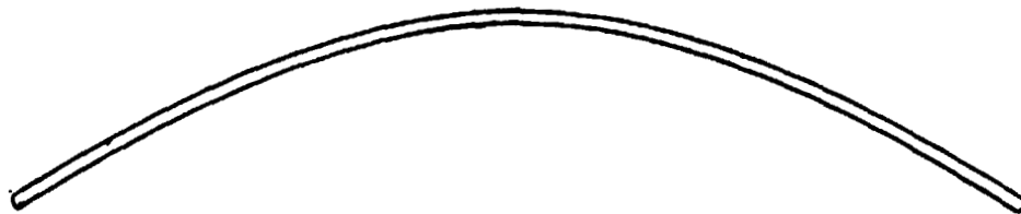
(b) Parabolic bow simulating thermal distortion
