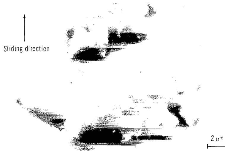
(b) Thin film and wear debris of tungsten transferred to HPF.
