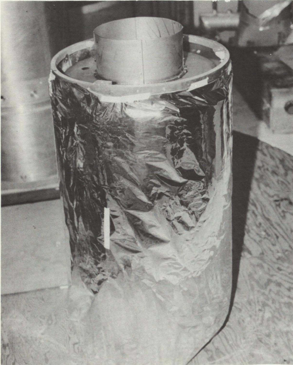
Figure 72: Dewar Heat Exchangers
