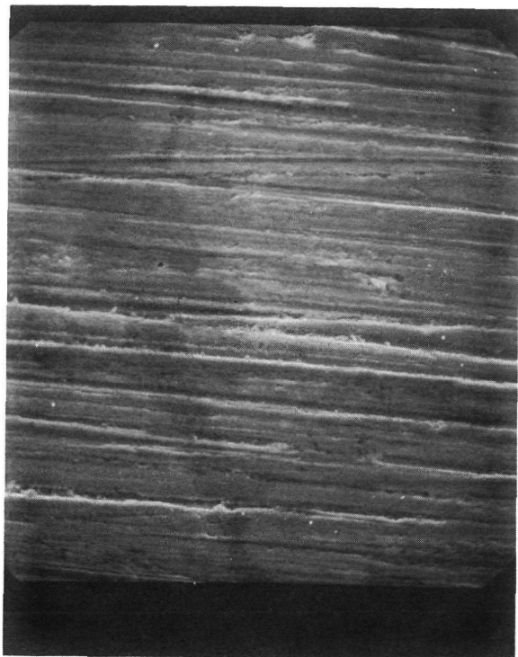
(a) As-machined copper surface. X1000.
