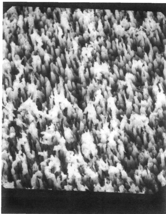
(c) Sputtered copper surface having needle-like protuberances.
