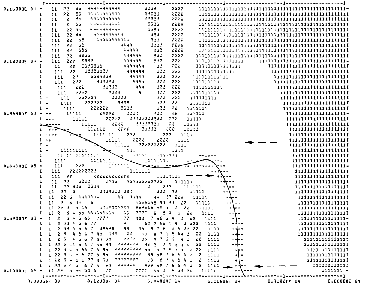
Figure 2.3.8. Normalized mean radial velocity contours as a function of z and R for an axisymmetric gust front with a 2000 m radius downdraft at t = 200 sec. [See figure 2.3.2 for explanation of notation.]
