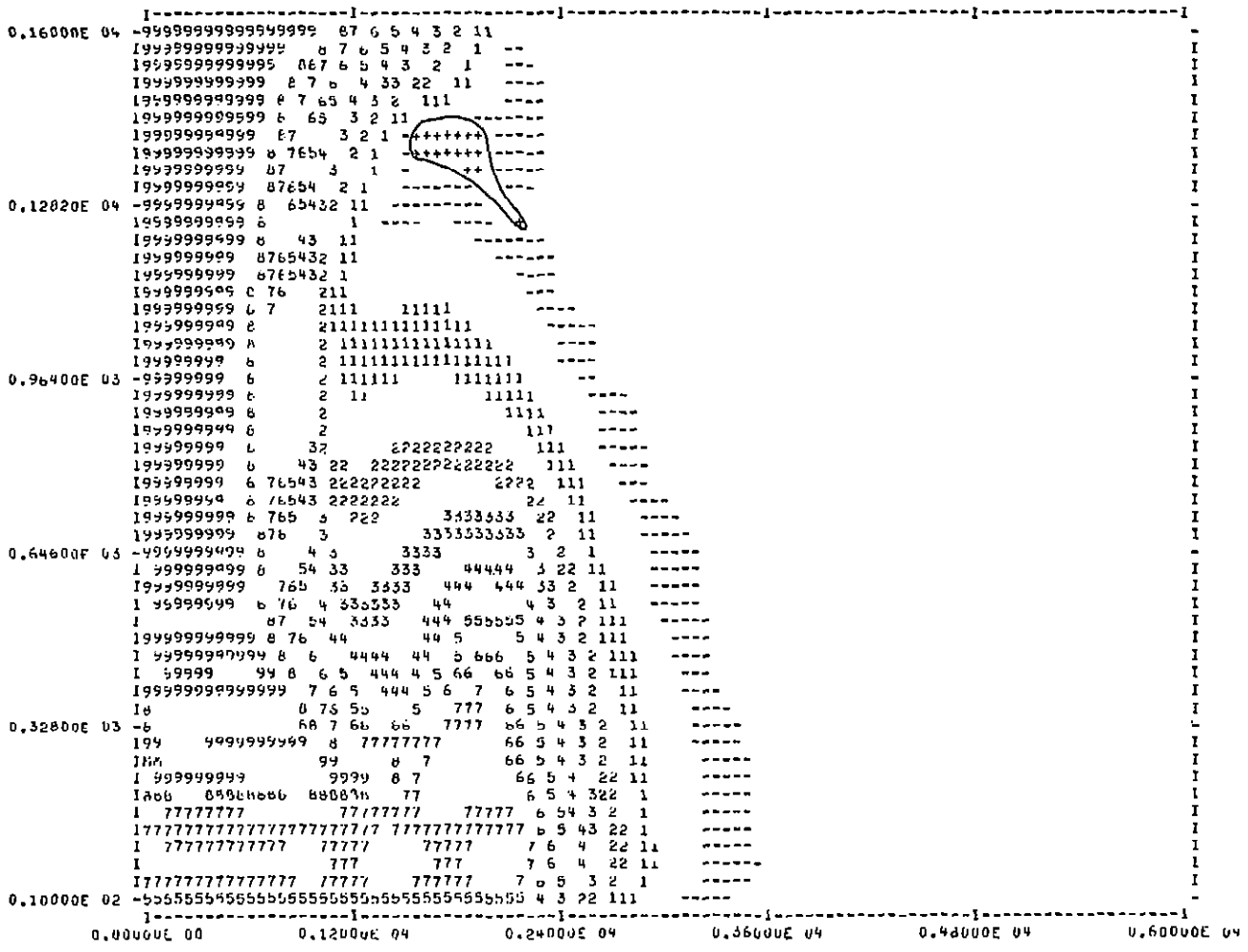
Figure 2.3.2. Normalized temperature contours as a function of z and R for an axisymmetric gust front with a 2000 m radius downdraft at t = 200 sec. [The numbers represent the percentage of the maximum value indicated across the top. The same number may represent either a + value. The P represents a positive maximum and M as minimum. The zero contour is outlined.]
