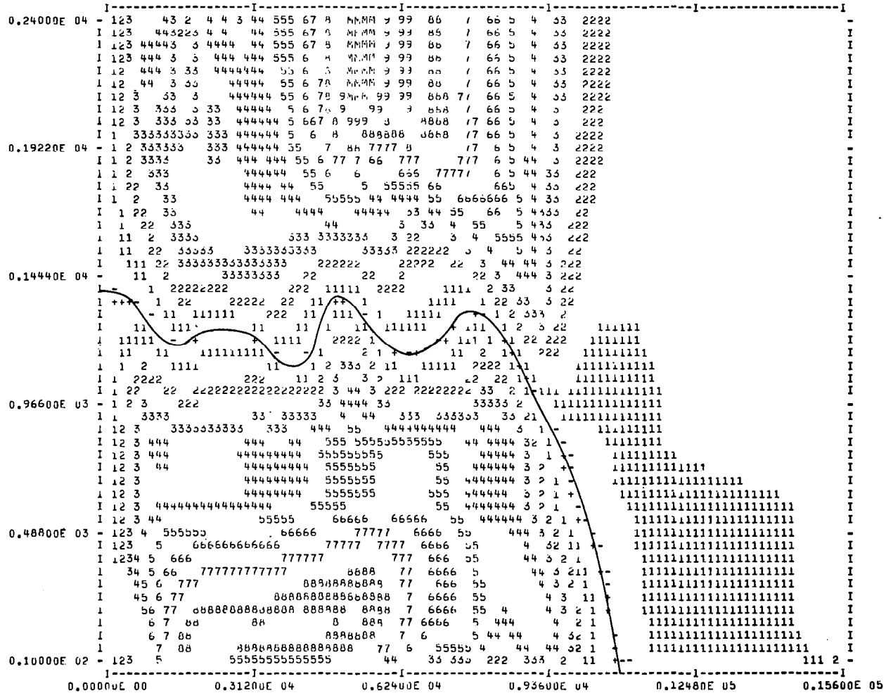
Figure 4.4.4. Normalized mean radial velocity contours as a function of z and y for a two-dimensional gust front with a 2000 m radius downdraft at t = 1000 sec. [See figure 2.3.2 for explanation of notation.]
