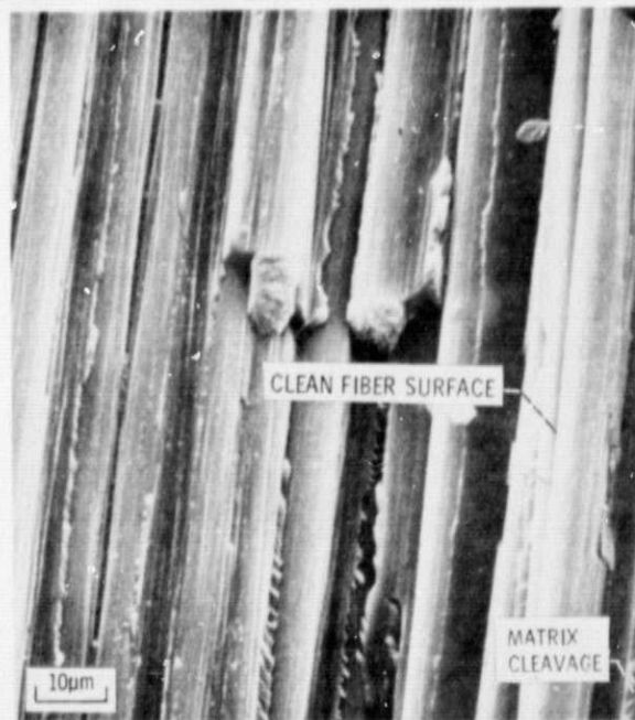
(c) ENLARGEMENT OF DETAIL IN (b) TO SHOW FRACTURE MODE.
