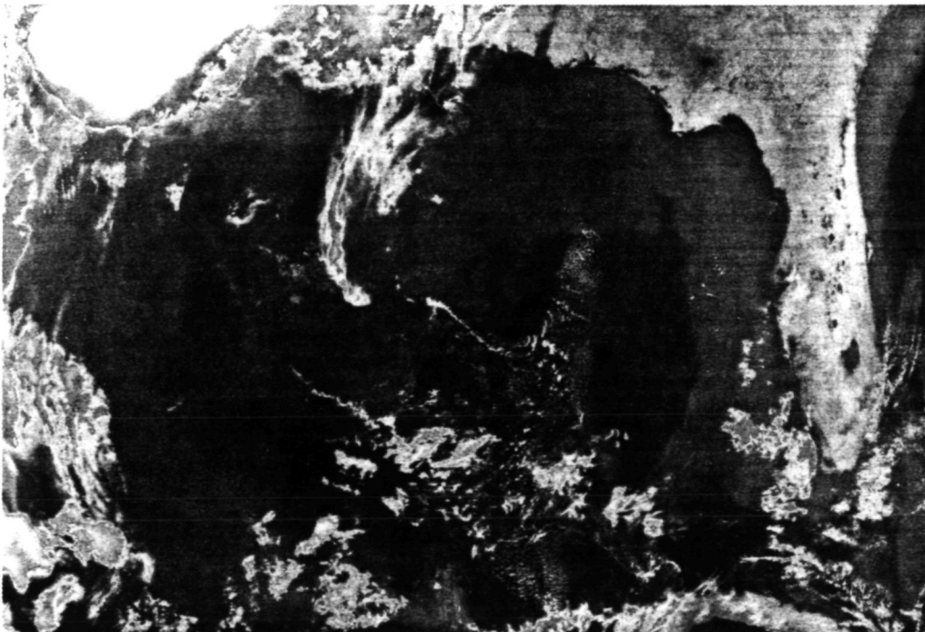
FIGURE 10. NOAA-3 INFRARED IMAGE, ORBIT 11085, 19 APRIL 1976, 0158Z. Warming of shallow regions along the Florida coast; evidence of positive heat flux along the inner shelf.
