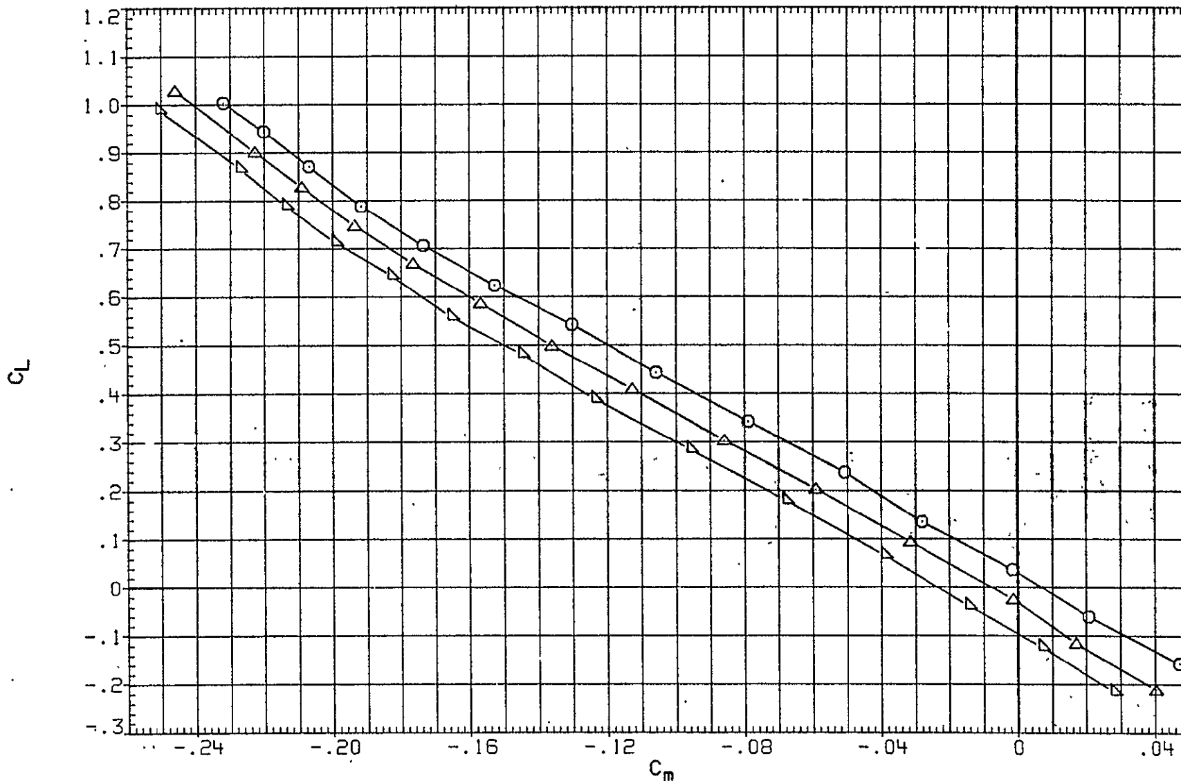
FIG. 4 EFFECT OF L.E. FLAP DEFL. FOR SIMPLE HINGE AND CONFORMAL FLAPS. TAIL OFF.
